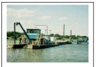
Hydraulic dredging: large cutterhead barge
