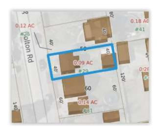
A site plan illustrating the setbacks from the property line to the existing and proposed structures on the site and the distance between existing and proposed structures on the site.
